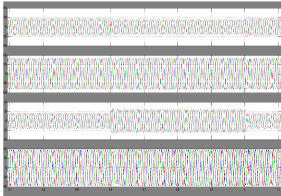
Fig12 (a) Source voltages. (b) Terminal voltages. (c) Voltage at the dc bus. (d) Compensator rms current in the proposed method.
