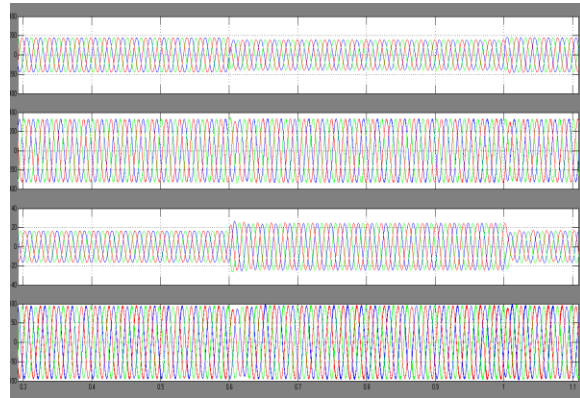
Fig12 (a) Source voltages. (b) Terminal voltages. (c) Voltage at the dc bus. (d) Compensator rms current in the proposed method.
