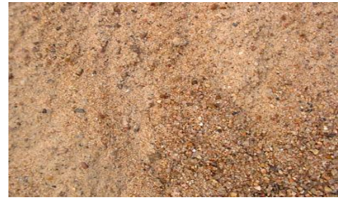
Figure 3.3 River sand used in concrete mixes
