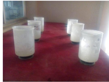
Figure 3.7 Water in 1 liter beaker placed on magnets
