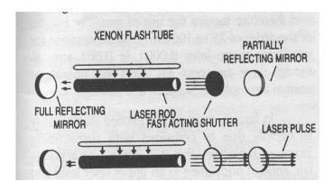
There are several ways of blocking and unblocking the optical paths between the mirrors. Different types of Q-switches like rotating prism, polarizing device, and dye solutions are employed. The tremendous energy released in this way can pierce through not only thick metallic plates but also the hardest material like diamond.
