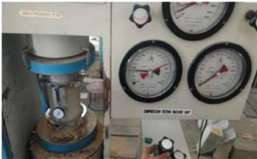
Fig 4.5 Testing of Cylinders-Modulus of Elasticity
