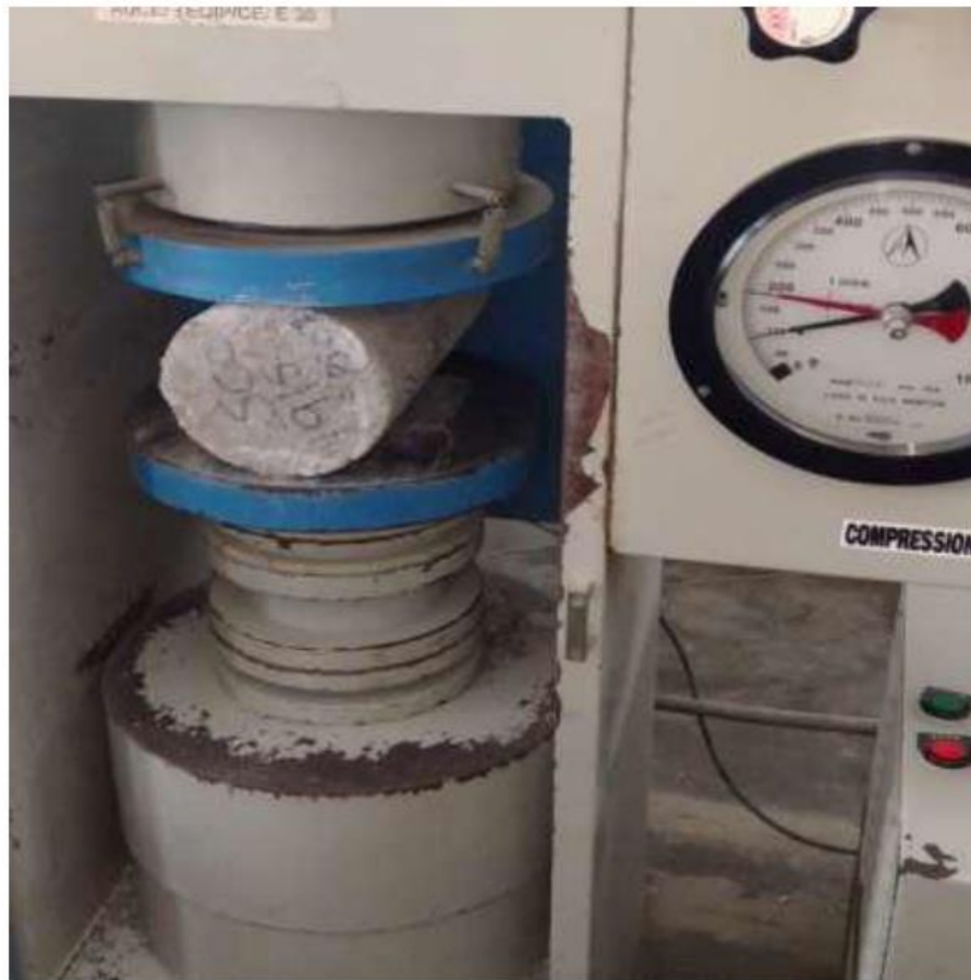
Fig.4.4 Testing of Cylinders- Split Tensile strength
