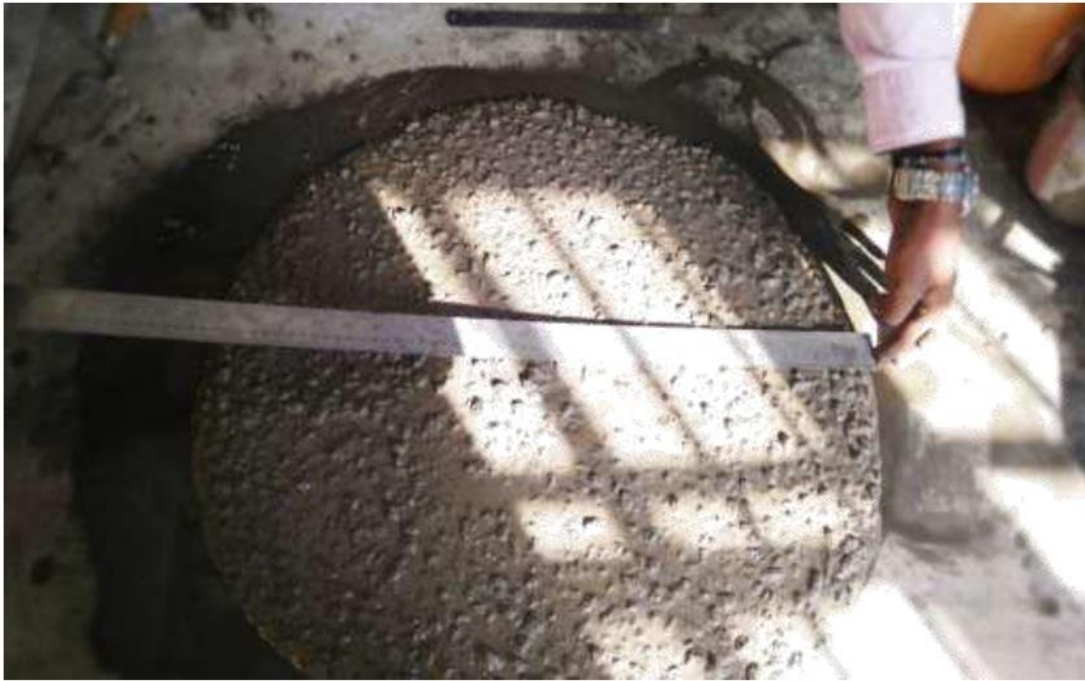
Fig. 4.2 Slump Flow test of SCC Mix
