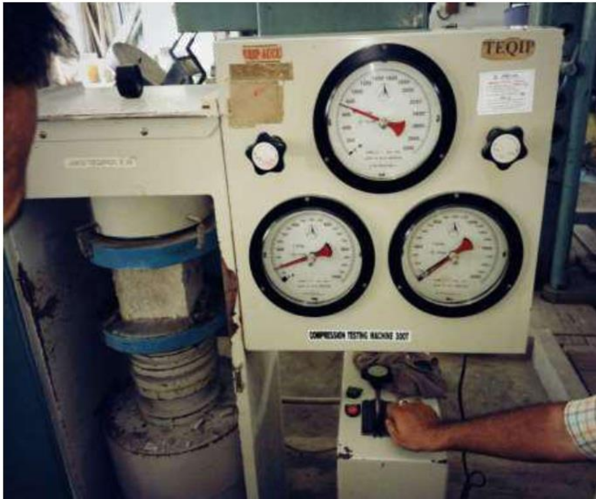
Fig 4.3 Testing of Cubes – Compressive Strength
