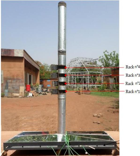
Fig. 1. Solar tower dryer
