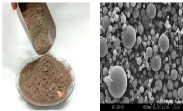
Fig.1 The original picture and SEM picture of Pond Ash (University of Kentucky Centre for Applied Energy Research)
