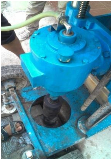
Figure 3.7 Core cutting equipment
