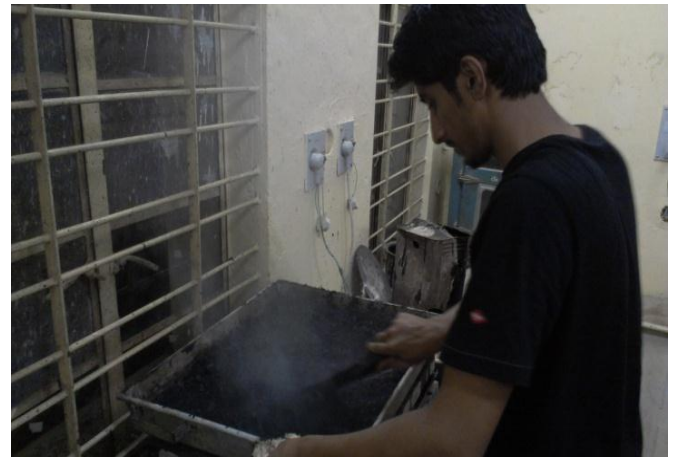
Figure three.3 Mixing of aggregates and binder for guidance of sample
