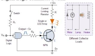
The base resistor, Rb is required to limit the output current from the logic gate.
