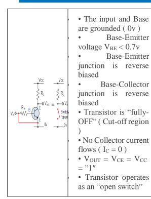
Then we can define the "cut-off region" or "OFF mode" when using a bipolar transistor as a switch as being, both junctions reverse biased,  $V_B < 0.7 v$  and  $I_C = 0$ . For a PNP transistor, the Emitter potential must be negative with respect to the Base.
