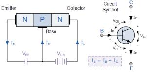
The most commonly used transistor configuration is the **NPN Transistor**. We also learnt that the junctions of the bipolar transistor can be biased in one of three different ways – **Common Base**, **Common Emitter** and **Common Collector**.
