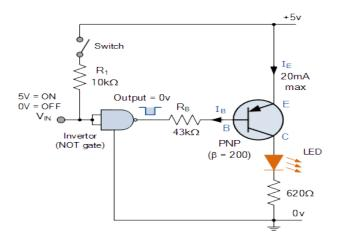
The equations for calculating the Base resistance, Collector current and voltages are exactly the same as for the previous NPN transistor switch. The difference this time is that we are switching power with a PNP transistor (sourcing current) instead of switching ground with an NPN transistor (sinking current).
