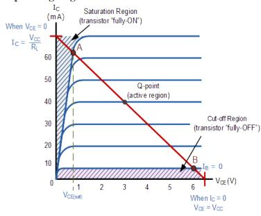
The pink shaded area at the bottom of the curves represents the "Cut-off" region while the blue area to the left represents the "Saturation" region of the transistor. Both these transistor regions are defined as:
