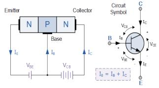
(Note: Arrow defines the emitter and conventional current flow, "out" for a Bipolar NPN Transistor.)
