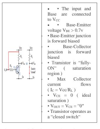
Then we can define the "saturation region" or "ON mode" when using a bipolar transistor as a switch as being, both junctions forward biased,  $V_B > 0.7v$  and  $I_C = Maximum$ . For a PNP transistor, the Emitter potential must be positive with respect to the Base.
