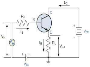
The common emitter configuration has a current gain approximately equal to the  $\beta$ value of the transistor itself. In the common collector configuration the load resistance is situated in series with the emitter so its current is equal to that of the emitter current.
