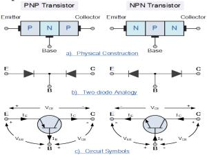
The construction and circuit symbols for both the PNP and NPN bipolar transistor are given above with the arrow in the circuit symbol always showing the direction of "conventional current flow" between the base terminal and its emitter terminal. The direction of the arrow always points from the positive P-type region to the negative N-type region for both transistor types, exactly the same as for the standard diode symbol.
