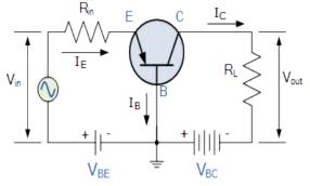
diodes back-to-back, this will give us two PN-junctions connected together in series that share a common **P** or **N** terminal. The fusion of these two diodes produces a three layer, two junction, three terminal device forming the basis of a **Bipolar Junction Transistor**, or **BJT** for short.
