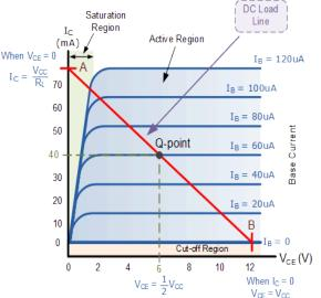
The most important factor to notice is the effect of Vce upon the collector current Icwhen Vce is greater than about 1.0 volts. We can see that Ic is largely unaffected by changes in Vce above this value and instead it is almost entirely controlled by the base current, Ib. When this happens we can say then that the output circuit represents that of a "Constant Current Source".
