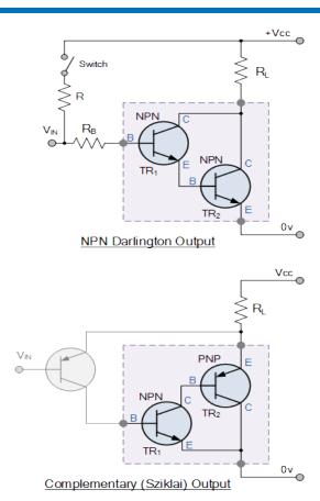
The above NPN Darlington transistor switch configuration shows the Collectors of the two transistors connected together with the Emitter of the first transistor connected to the Base terminal of the second transistor therefore, the Emitter current of the first transistor becomes the Base current of the second transistor switching it "ON".
