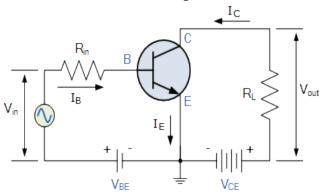
In this type of configuration, the current flowing out of the transistor must be equal to the currents flowing into the transistor as the emitter current is given as Ie = Ic + Ib.
