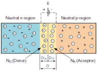
As the N-type material has lost electrons and the P-type has lost holes, the N-type material has become positive with respect to the P-type. Then the presence of impurity ions on both sides of the junction cause an electric field to be established across this region with the N-side at a positive voltage relative to the P-side. The problem now is that a free charge requires some extra energy to overcome the barrier that now exists for it to be able to cross the depletion region junction.
