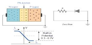
The potential barrier that now exists discourages the diffusion of any more majority carriers across the junction. However, the potential barrier helps minority carriers (few free electrons in the P-region and few holes in the N-region) to drift across the junction.
