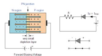
This condition represents the low resistance path through the PN junction allowing very large currents to flow through the diode with only a small increase in bias voltage. The actual potential difference across the junction or diode is kept constant by the action of the depletion layer at approximately 0.3v for germanium and approximately 0.7v for silicon junction diodes.
