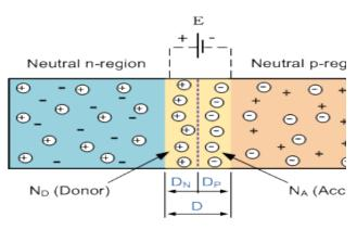
This is all well and good, but these newly doped N-type and P-type semiconductor materials do very little on their own as they are electrically neutral. However, if we join (or fuse) these two semiconductor materials together they behave in a very different way merging together and producing what is generally known as a "PN Junction".
