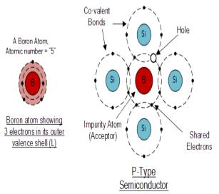
The diagram above shows the structure and lattice of the acceptor impurity atom Boron.
