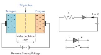
This condition represents a high resistance value to the PN junction and practically zero current flows through the junction diode with an increase in bias voltage. However, a very small leakage current does flow through the junction which can be measured in microamperes, (µA).
