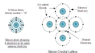
The diagram above shows the structure and lattice of a 'normal' pure crystal of Silicon.
