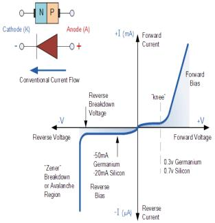
But before we can use the PN junction as a practical device or as a rectifying device we need to firstly **bias** the junction, ie connect a voltage potential across it. On the voltage axis above, "Reverse Bias" refers to an external voltage potential which increases the potential barrier. An external voltage which decreases the potential barrier is said to act in the "Forward Bias" direction
