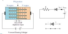
However, if we were to make electrical connections at the ends of both the N-type and the P-type materials and then connect them to a battery source, an additional energy source now exists to overcome the potential barrier.
