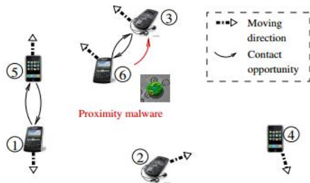
Fig. 1. Proximity malware propagation. Malware can propagate through bluetooth connections when two nodes are in geographical proximity.
