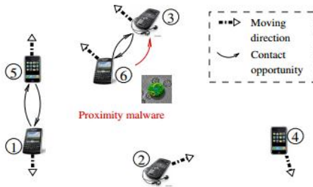
Fig. 1. Proximity malware propagation. Malware can propagate through bluetooth connections when two nodes are in geographical proximity.
