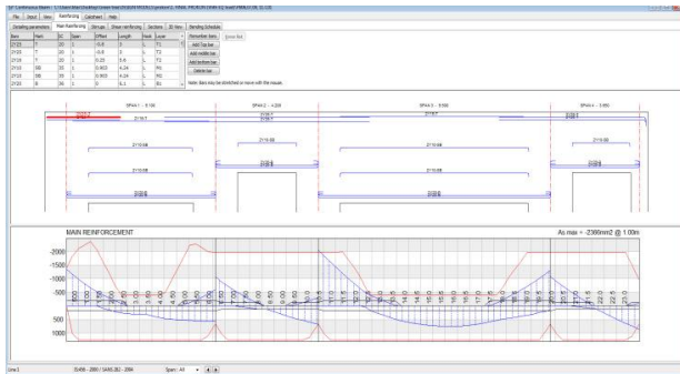
Fig 11: Design of beam for flexure
