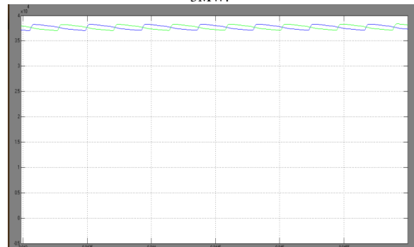
Fig.8.Simulation waveform of the output filter Capacitor Voltages (VC1 and VC2).
