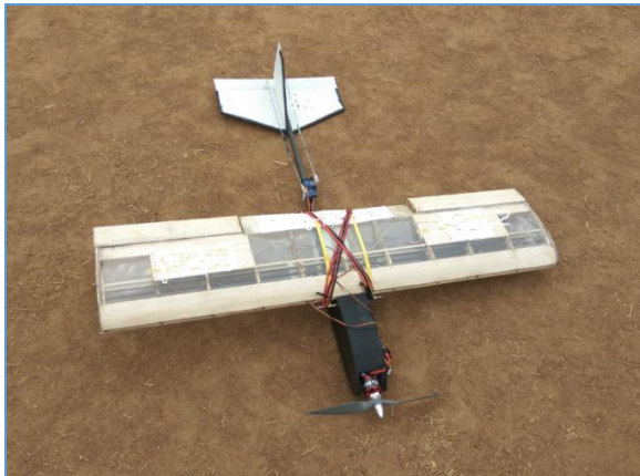
Figure 4. Final model aircraft constructed using the 3D printed fuselage.
