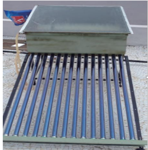
Fig.1 Experimental set up of double basin solar still with evacuated tubes
