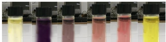
Figure 1. Colour of solutions (from left to right): AgNPs, AgNPs+ 10^{-2}M Cr (VI), AgNPs+ 10^{-4}M Cr(VI), AgNPs+ 10^{-6}M Cr(VI), AgNPs+ 10^{-9}M Cr(VI), AgNPs+ 10^{-12}M Cr(VI)
