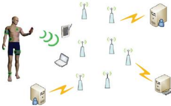
Fig. 4 Inter-BAN communication architecture: ad hoc based mode
