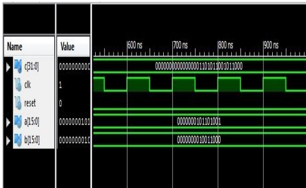
Fig. 12 Simulation result for Dadda Multiplier
