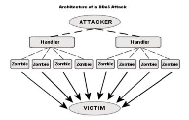
DDoS attacks last for a period of time for exhausting the server resources, such as CPU, memory, and connection capacity by the following types of attacks: Session Flooding Attacks, Request Flooding Attacks, Asymmetric Attacks, Slow Request/Response Attacks, Among the above attacks, DDoS attack is the most prevalent threat in cyberspace. Researchers have been proposing many defence mechanisms to combat the attacks.
