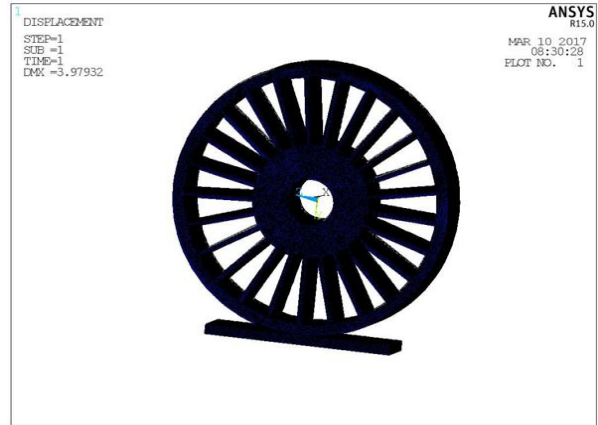
Fig 4.4 Deflection for load of 4000N
