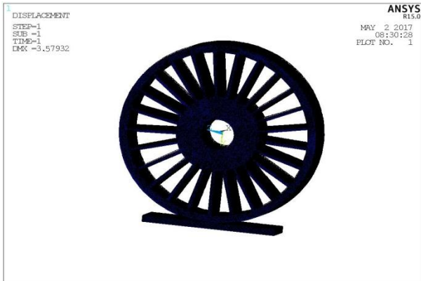
Fig 4.1 Deflection for load of 3500N
