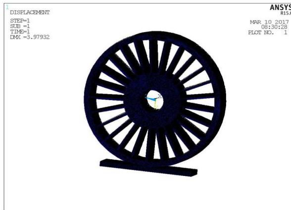
Fig 4.4 Deflection for load of 4000N
