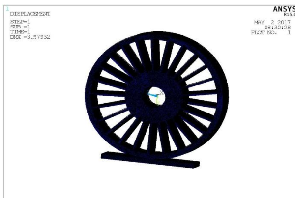
Fig 4.1 Deflection for load of 3500N
