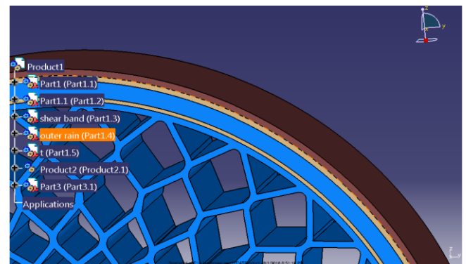
Fig 3.3 Model of NPT with honey comb lattice structure in CATIA
