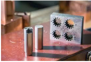
Fig. 1.8 various shapes cut with wire cut EDM
