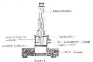
Table 1. Table example. In an ultrasonic interferometer, the ultrasonic waves are produced by the piezoelectric effect method. In a fixed frequency variable path interferometer, the wavelength of the sound in an experimental liquid medium is measured, and from this one can calculate its velocity through that medium. The apparatus consists of an ultrasonic cell, which is a double walled brass cell with chromium plated surfaces having a
