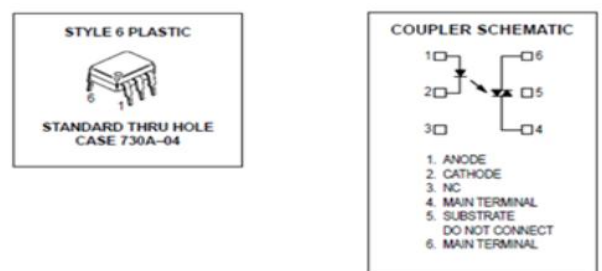
Fig.5: MOC3021 pin configuration
