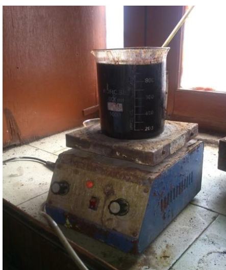
Figure – 2.3 Heating of Neem oil by Magnetic Stirrer Heater
