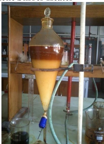
Figure –2.4 Washing of NOME in a separating funnel
