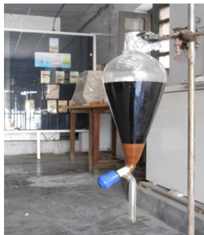
Figure – 2.5 Separation of NOME and Glycerol
