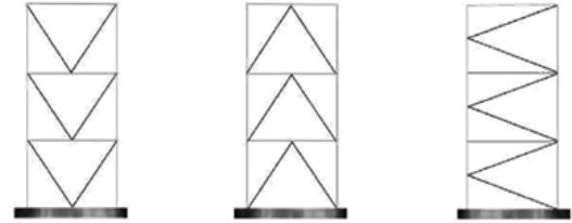
Examples of bracing schemes for concentrically braced frames: X braced; diagonally braced; alternative diagonally braced; V braced; inverted V-braced; and K-braced
