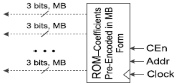
Fig. 2.5. The ROM of pre-encoded multiplier with standard coefficients in MB Form.
