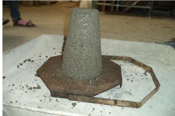
Fig shows slump test on RAC
