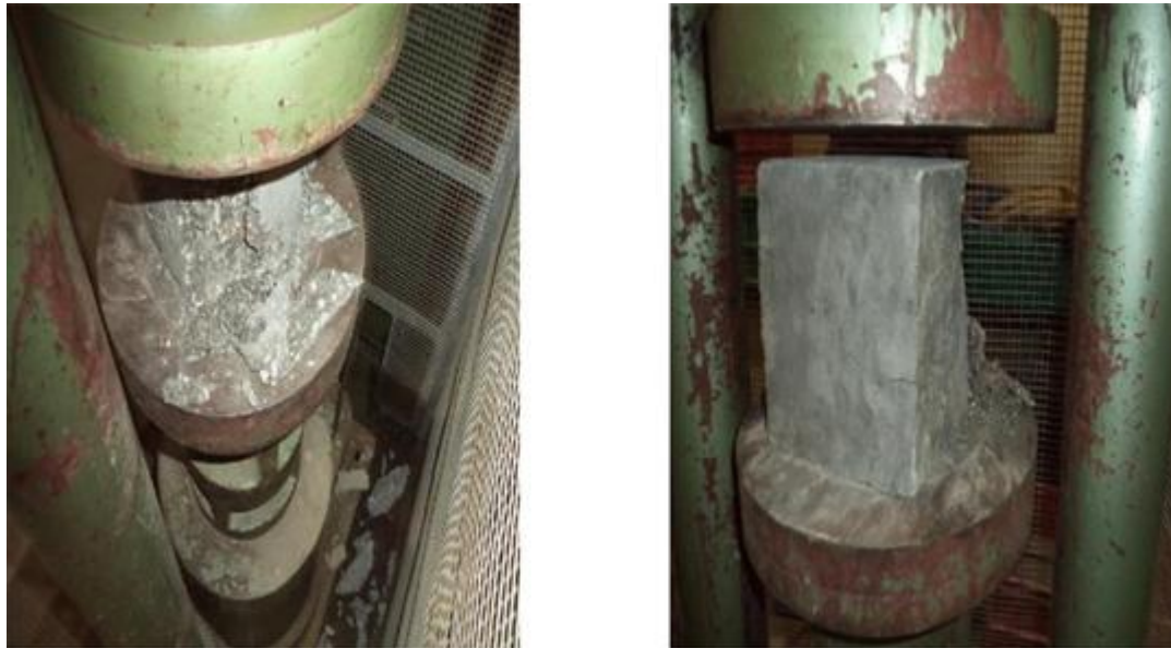
Fig shows compression test on cubes and crushed on the specimen
